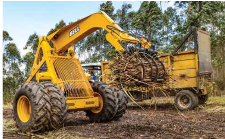
All Bell Tri-wheeler derivatives – a cane loader, a logger, a forklift and the Versalift – feature a ROPS- and FOPS-certified frame and a water-cooled Yanmar engine to deliver a low-noise, fuel-efficient and highly manoeuvrable machine solution.
