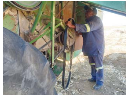
John Ngwenya had to replace the drive belt on his combine. He uses the combine to shell the maize. He was still busy picking up maize that was scattered after a tornado swept through his lands.
