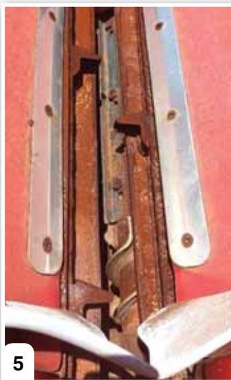
5 The deck plates, gathering chain and snapper rollers of the maize header.
